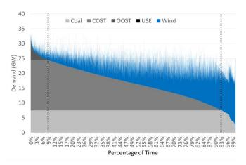
Note that anomalies in the right hand side of the wind generation curve are present in the original wind data collected from operating wind farms, and are thought to be due to curtailment during low demand periods.
