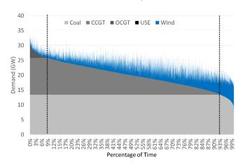
Figure IV.3 - Least cost optimized results for High Wind Scenario (25GW wind installed)
