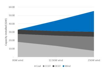
Figure IV.4 - Least cost optimized capacity of each technology installed in each wind scenario
